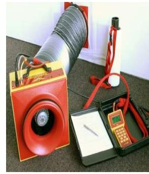
Duct Pressure Testing for Air Leakage
