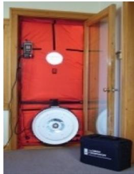
Blower Door Testing for Air Infiltration
