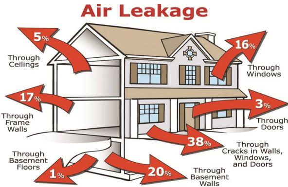
Drawing courtesy of Touch 'n Foam Insulating Sealants
